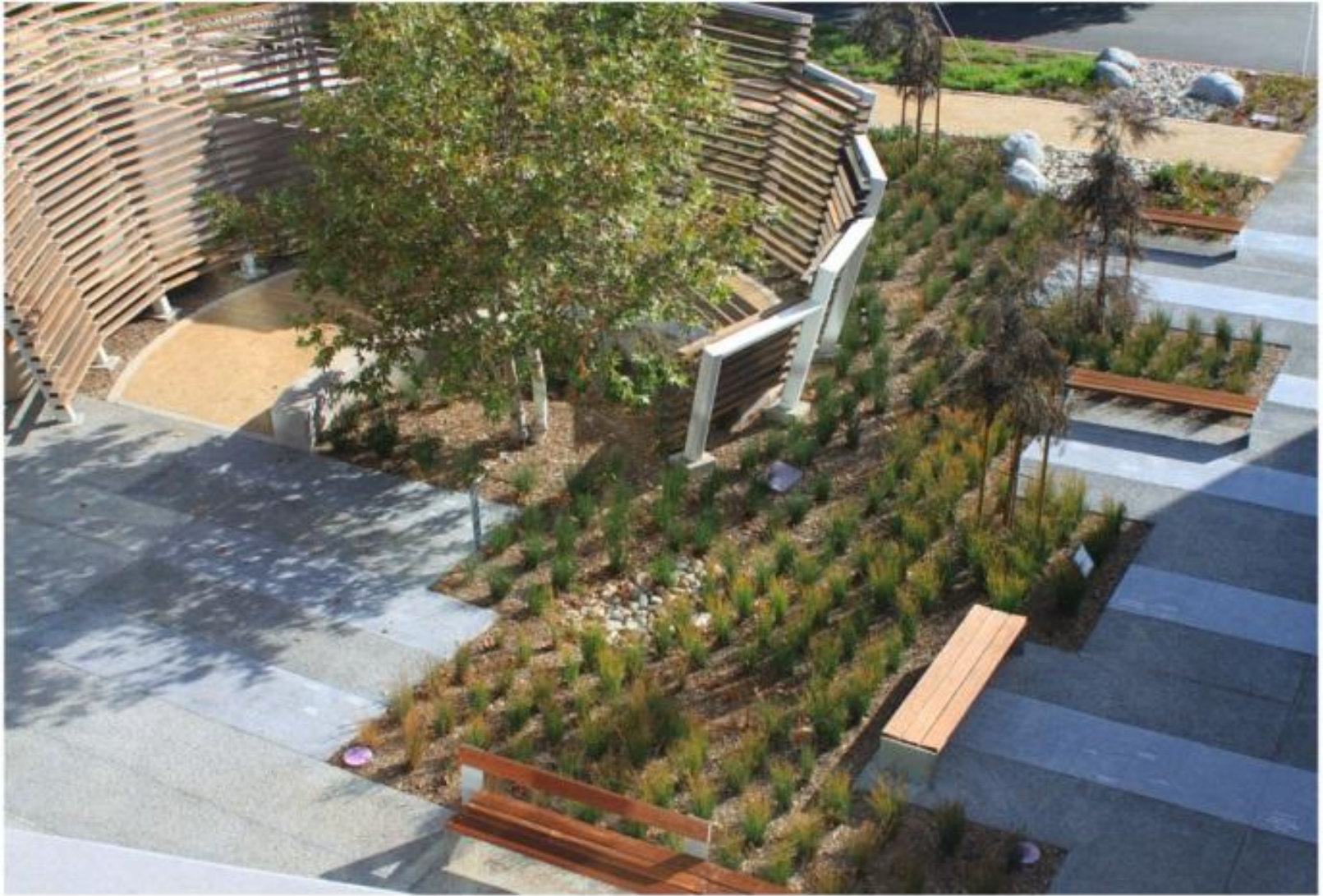
The central courtyard includes a small outdoor classroom and rain garden that treats roof runoff before it enters the cistern. The wooden screen shading the north wing was made from repurposed wine barrels donated by a local winery.
