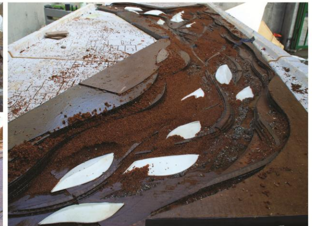
MODEL AFTER WATER TEST RESULTANT SAND SCOURING AND DEPOSITION
