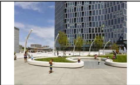
The pre-cast concrete bench at the lawn retains the grass mound and supports an interactive water feature. The floor can be flooded with a splash pad and a channel of water traces the top of the bench.
